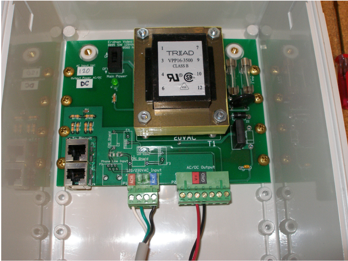
Fig 1.9 Inside look at the external transformer box.
